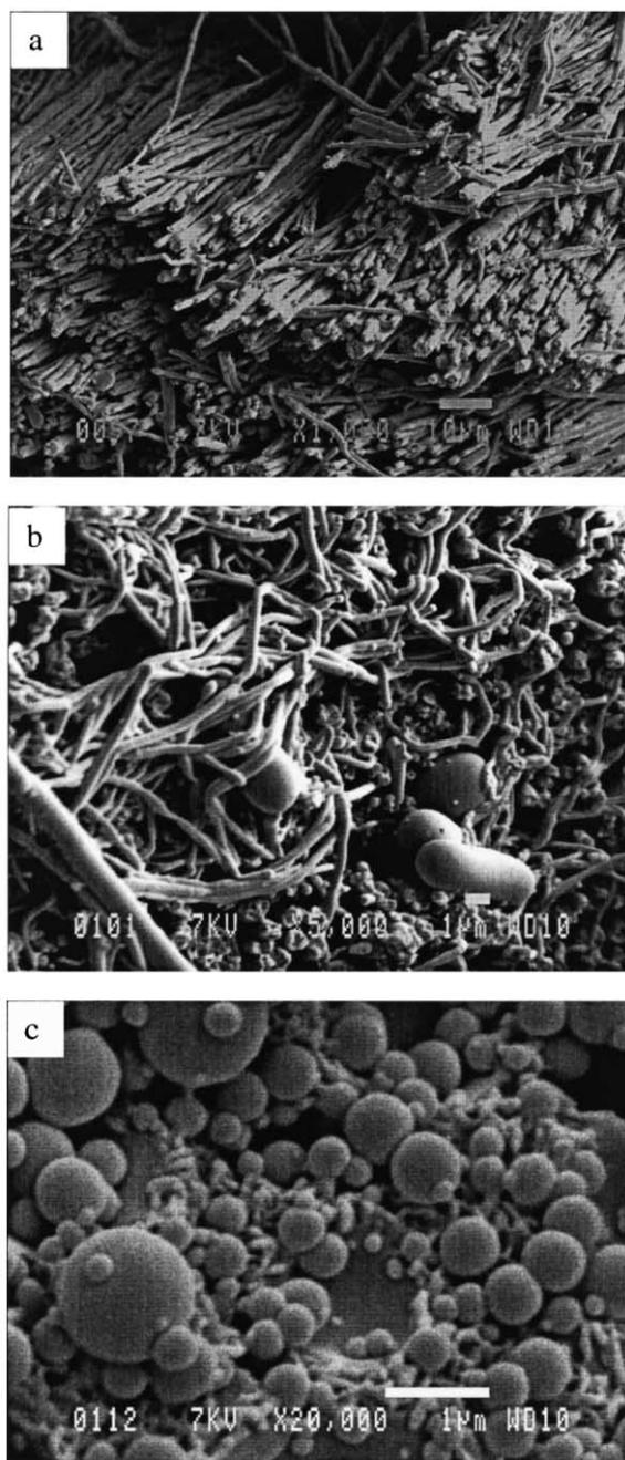
Fig. 8. SEM micrographs after removal of the PS phase from 40/60 PC/PS blend of the first-melt extrusion at three different radial positions: (a) at the periphery; (b) at the midpoint; (c) at the centre.
