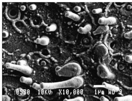
Fig. 9. SEM micrographs for 20/80 PC/PS blend obtained from the cryogenically fractured cross-section surfaces of the re-melt extrusion.
