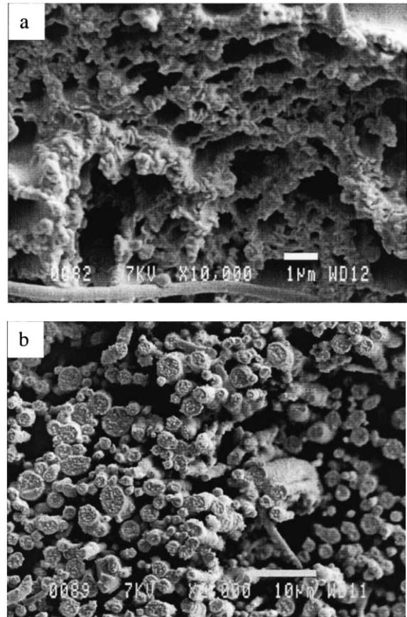
Fig. 3. SEM micrographs after removal of the PS phase from 50/50 PC/PS blend: (a) first-melt extrusion blend; (b) second-melt extrusion blend.
