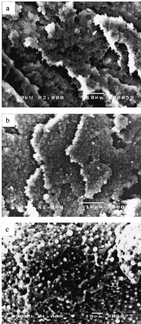
Fig. 6. SEM micrographs for 50/50 PC/PS blend obtained from the cryogenically fractured cross-section surfaces: (a) first-melt extrusion blend; (b) second-melt extrusion blend; (c) third-melt injection blend.
