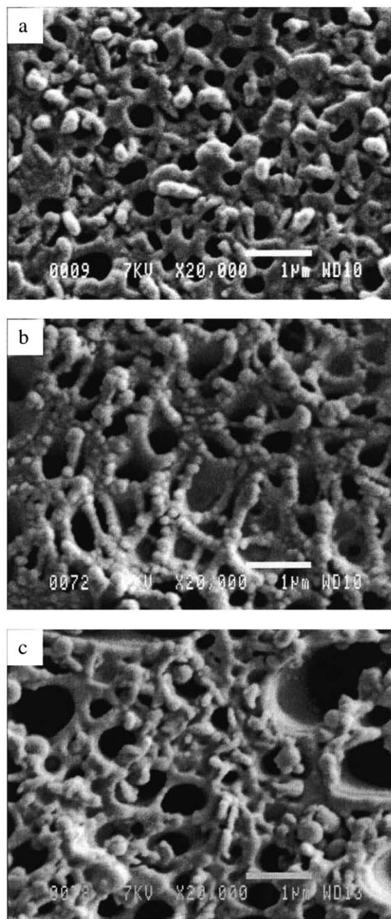
Fig. 1. SEM micrographs after the removal of the PS phase from 80/20 PC/PS blend: (a) first-melt extrusion blend; (b) second-melt extrusion blend; (c) third-melt injection blend.
