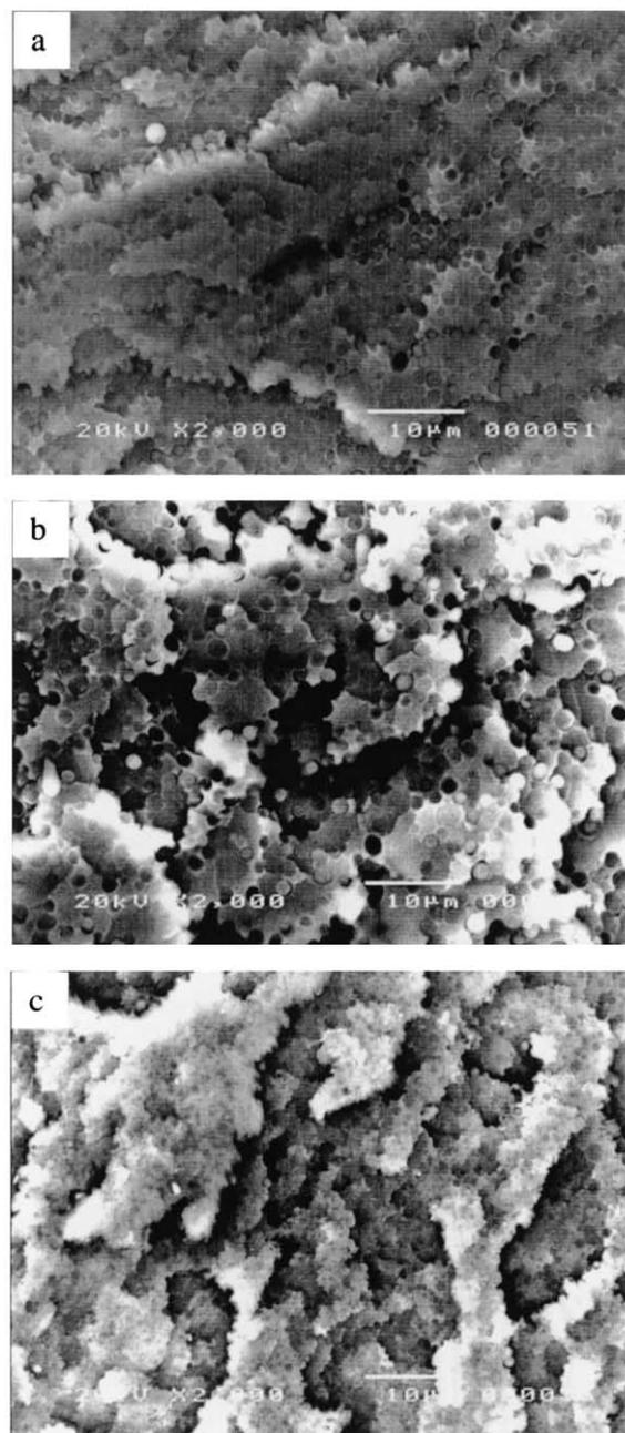
Fig. 5. SEM micrographs for 80/20 PC/PS blend obtained from the cryogenically fractured cross-section surfaces: (a) first-melt extrusion blend; (b) second-melt extrusion blend; (c) third-melt injection blend.
