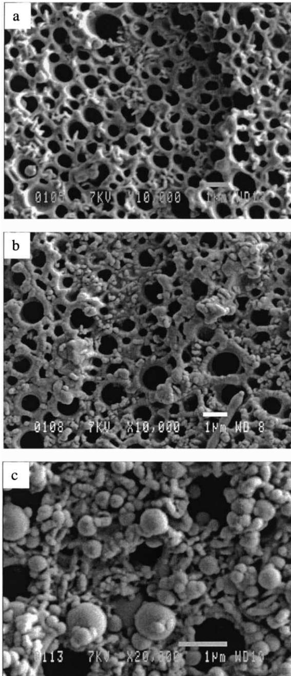
Fig. 2. SEM micrographs after removal of the PS phase from 60/40 PC/PS blend: (a) first-melt extrusion blend; (b) second-melt extrusion blend; (c) third-melt injection blend.
