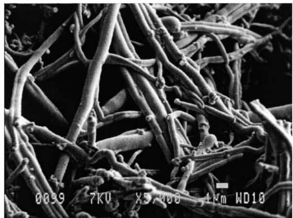
Fig. 4. SEM micrographs after removal of the PS phase from 40/60 PC/PS blend of the first-melt extrusion.
