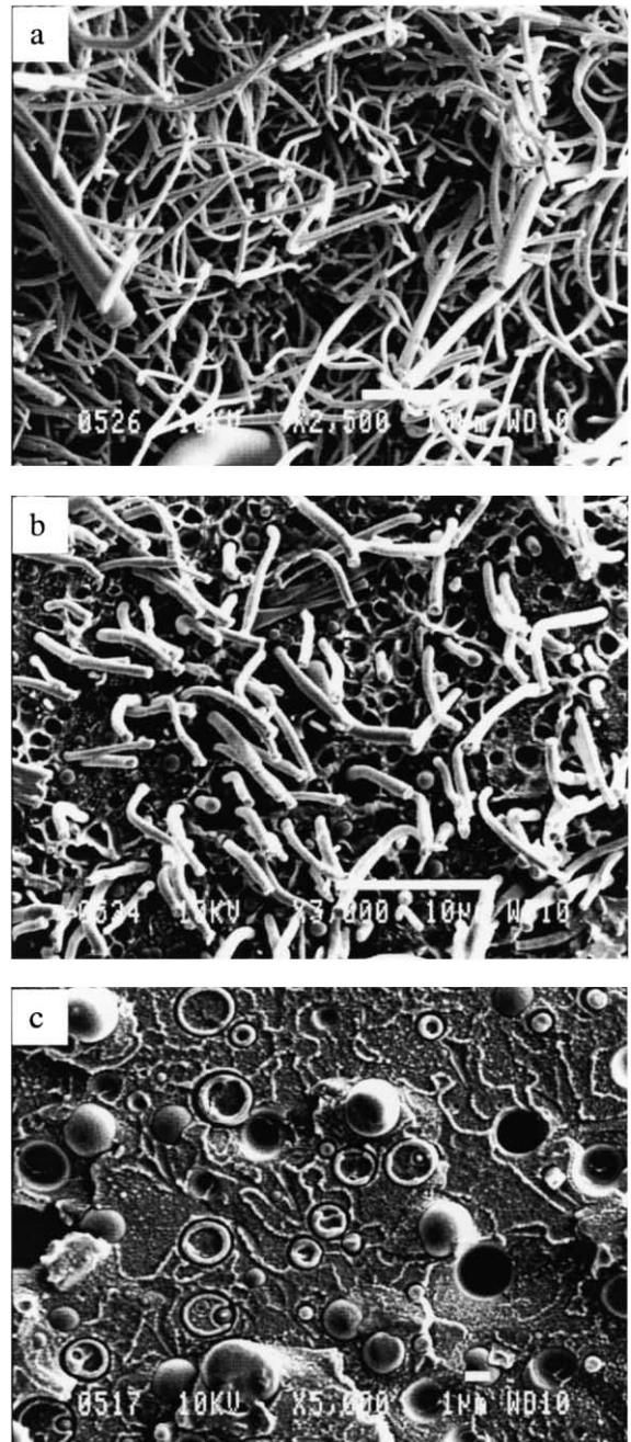
Fig. 7. SEM micrographs for 80/20 PC/PS blend obtained from the cryogenically fractured cross-section surfaces of the first-melt extrusion at three different radial positions: (a) at the periphery; (b) at the midpoint; (c) at the centre.
